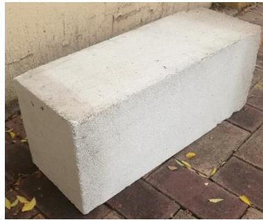
(b): Lightweight concrete
