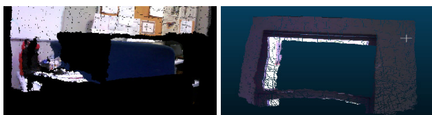
FIGURE 5. The leftmost image depicts the shadow effect issue of the structured light and time-of-flight sensors. The rightmost image shows another problem with these sensors, which is the incompatibility with specular surfaces.
