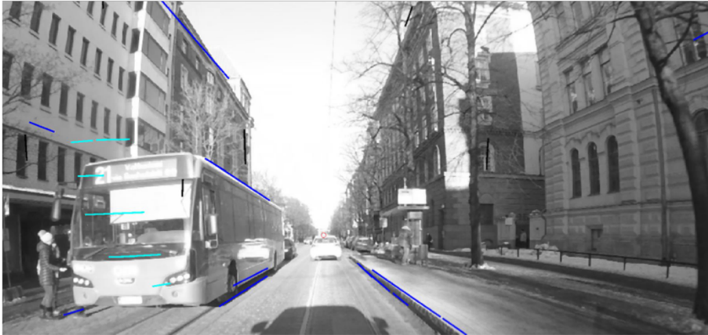
Figure 1: Example of vanishing points representation, determined in urban environment. Horizontal (turquoise) and along the direction of propagation (blue) lines. Central vanishing point (red dot).
