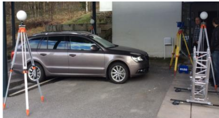
Figure 3. The car was scanned by a FARO Focus3D X330 terrestrial laser scanner. The scanner was mounted on the yellow tripod, seen near the right. Three of the five white reference spheres are also visible.
