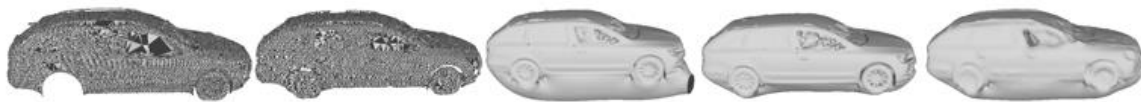
Figure 12. Car reconstruction from different point densities by the methods of the Crust and SPR. Left two images: the Crust with the resampling points of 0.01 m and 0.05 m, respectively; Right three images: the SPR with the original points and the resampling points of 0.01 m and 0.05 m, respectively.
