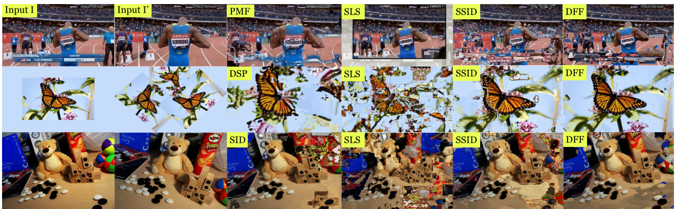
Figure 8. Image alignment results for the images of similar scene content but with significant geometric variations. Each algorithm warps the image I' onto the image I based on its estimated flow. The first test image pair was also used in [6], and SLS [6] cropped the area of high confidence matches to show. The last test image pair depicting a wide-baseline stereo case was used in [20]. Unlike [20], the epipolar geometry between the images is not assumed to be known here for a general image alignment task. (All figures are best viewed in color.)
