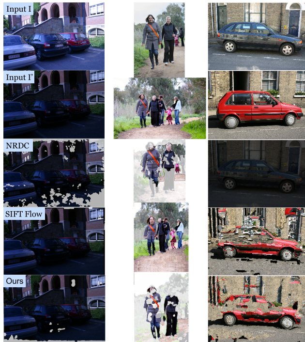
Figure 1. Some typical challenges of matching a pair of images. First two rows: two input images with significant photometric, geometric and scene content changes (from left to right). Third to fifth rows: image warping results from the second image to the first one using the estimated correspondences by NRDC [5], SIFT Flow [12], and our DFF method. DFF yields dense coherent matches consistently. NRDC gives no match for different scenes.
