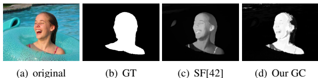
Figure 6. Example saliency detection results to demonstrate the limitation of precision recall analysis. When using precision recall analysis, the saliency map in (c) continually achieves near 100% precision for a wide range of recall values, while the saliency map in (d) performs worse because of the small number of false alarm foreground pixels in the upper left corner. However, the saliency map in (d) is closer to the ground truth (b) and better reflects the true salient region in the original image (a).
