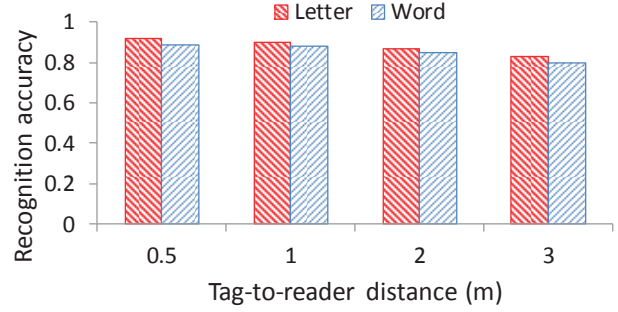
Figure 24— Impact of tag-to-reader distance.
