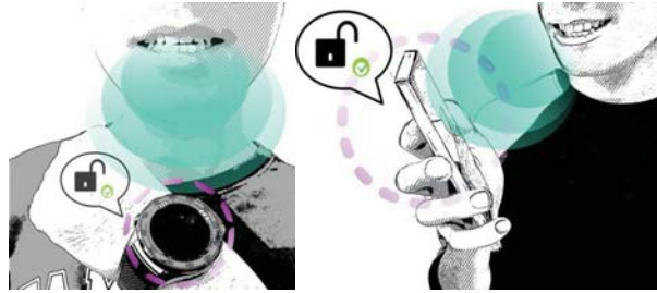
Fig. 1. Application scenarios of BiLock. A user places his/her smartphone or smartwatch 5 cm to 15 cm away to his/her lips, and performs an occlusion gesture. The microphone embedded in the smartphone or smartwatch records the sounds generated by the occlusion gesture and extracts features, which are fed into a classifier for user authentication. BiLock is able to achieve average FRR and FAR of 4.33% and 0.82% in presence of noise up to 50 ~ 60 dB (measured next to the device) in indoor environments.
