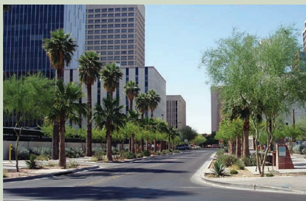
FIG. S1. Present-day streetscape (2nd Ave.) in downtown Phoenix, illustrating the influence of sustainable street-level shading. Previously, a single strip of palm trees provided little pedestrian shade. To increase thermal comfort and reduce daytime urban ambient temperatures, the Downtown Phoenix Plan recommended planting 1) a double row of broad canopy, low-water demand trees to increase shading and 2) low shrubs or screens to reduce pedestrian exposure to longwave radiation emitted from the adjacent asphalt road (Source: City of Phoenix 2008).
