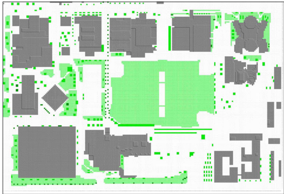
Fig. 3 Part of the area input file for ENVI-met simulations which was based on Figs. 1 and 2. Individual grid cell size was 2.5 \times 2.5 \times 5 m
