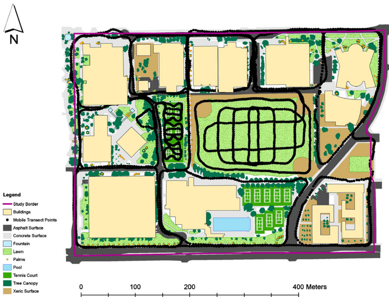
Fig. 2 Map of traverse route and classification of different surface types within the study area
