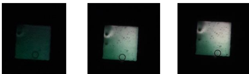
Figure 7. 15. Light emission at different applying voltages from the same device (from 4 V to 7 V).
