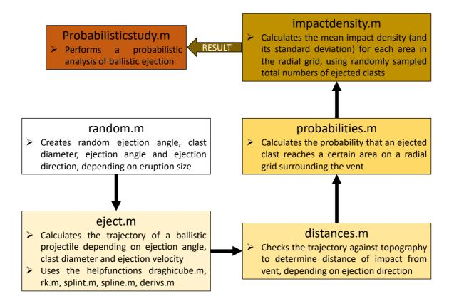
An example for the use of this workflow and a detailed description of the method can be found in Strehlow et al. (2017). The core-function is eject.m, which is a translation of the Visual Basic code of Eject! (Mastin, 2001; 2011) into Matlab.
