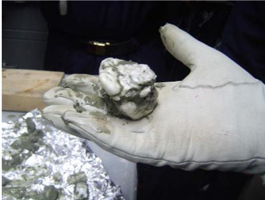
Figure 2: Sample of methane hydrate taken offshore Concepcion, Chile (840 meters below sea level), drilled by the research vessel Vidal Gormaz (Cruise VG04). Credit: FONDEF Project D04I1111.
