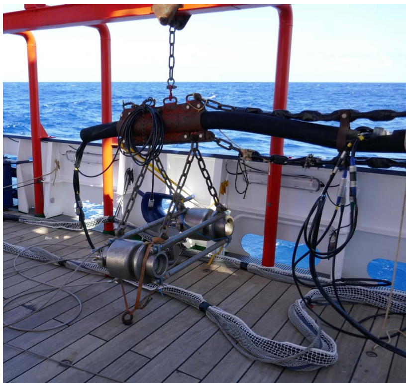
Figure 5.34 A cluster of two G-Guns used as seismic source. Photo credit: Wolfram Geissler.
