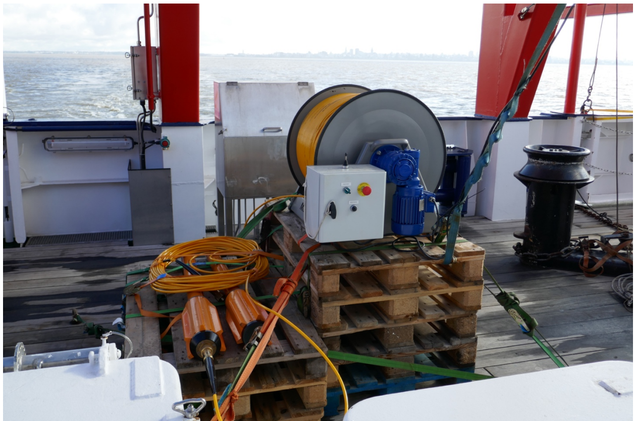
Figure 5.50 Magnetometer system (Marine Magnetics SeaSPY2™ longitudinal gradiometer). Photo credit: Wolfram Geissler.
