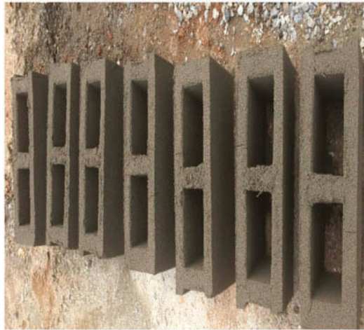
Plate 5. Sandcrete block produced from (SAD and RD).
