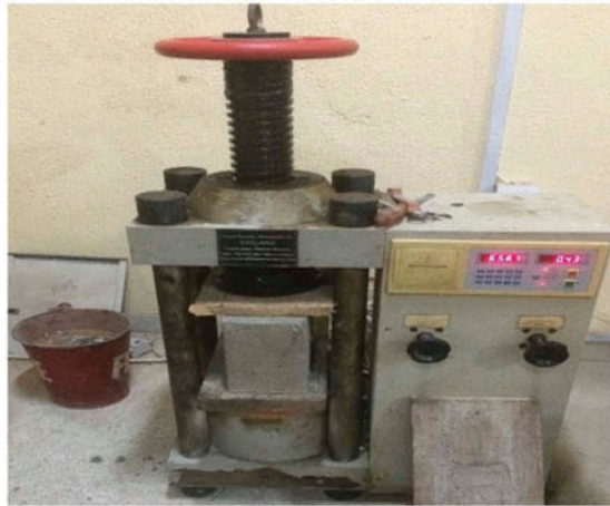
Plate 6. Compression testing machine loaded with sample.
