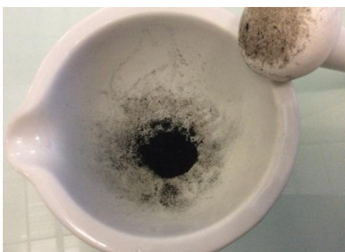
Fig. 2.11 Solid residue of the SCB acid extraction after drying and grinding.
