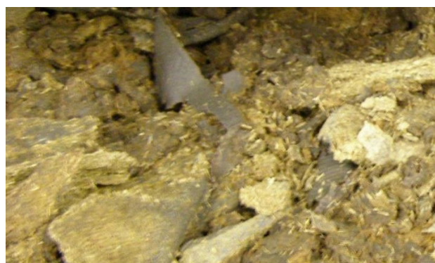
Fig. 2.8 Solid residue of the SCB acid extraction before drying and grinding.
