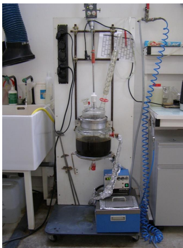
Fig. 2.5 Set-up for the alkaline extraction on SCB in a 4 L jacketed glass reactor.
