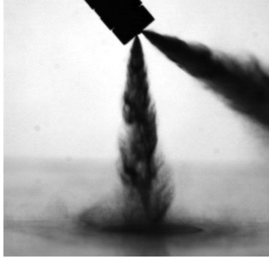
Figure 3.4: GDI spray impinging upon a smooth plate. Fuel pressure is 100bar.
