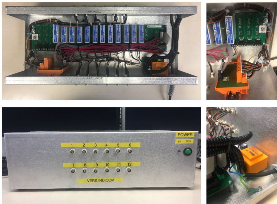
Figure 3.22: Top Left: Overview of the amplification system, in green the back-panel, in blue the amplification modules. Top Right: Break-out box. Bottom Left: Exit panel with BNC connections. Bottom Right: 5 V Power unit.
