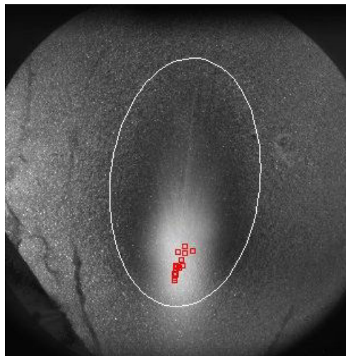
Figure 4.25: Evolution of ellipse focus position on time averaged image, the white area in the centre is the impingement area. Red squares present the position of the focus through time. White line displays the edge of the liquid film at the end of injection. Impingement angle is 60^\circ .
