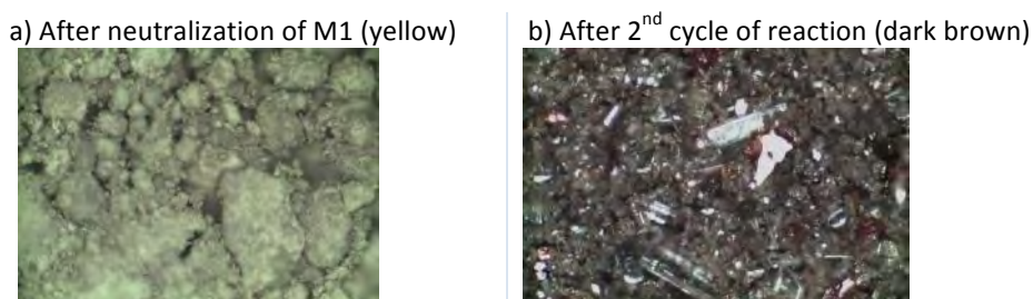
Figure 69. Optical microscopy (x10) of solid phase after adjustment to pH 5 with NaOH and after 2 nd cycle of reactions. Experimental conditions: \text{AgNO}_3/\text{K}_2\text{S}_2\text{O}_8 (1:1), \text{KH}_2\text{PO}_4/\text{K}_2\text{HPO}_4 (0.1:0.1 M), 100°C, 30 minutes
