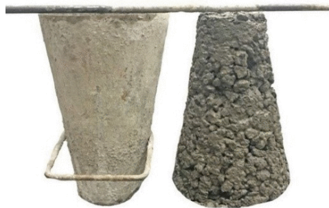
Figure 10. Slump test of C4 concrete with w/c 0.5, SP 0.6%; VMA 0.35%; and Vp/Vv 101%.
