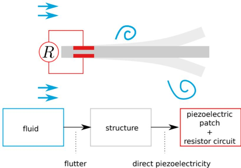
**Transform ambient fluid flow energy into electrical energy**
