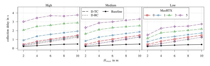
Figure 10: Total collection delay for different H<sub>max</sub> and MaxRTX values, and for different vehicular density scenarios (LuST).
