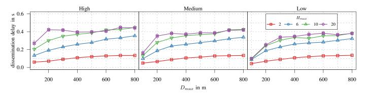
Figure 8: Mean dissemination delay for different  $D_{\text{max}}$  and  $H_{\text{max}}$  values, and for different vehicular densities (LuST).
