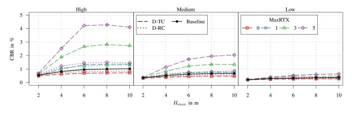
Figure 11: Mean CBR for different  $H_{\text{max}}$  and MaxRTX values, and for different vehicular density scenarios (LuST).
