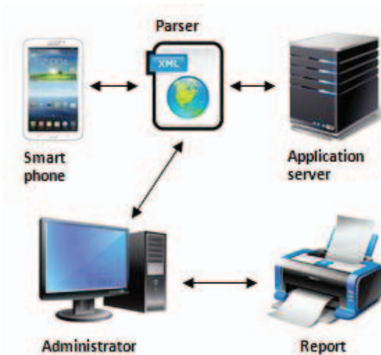
Fig. 2. Architecture of smartphone attendance system.
