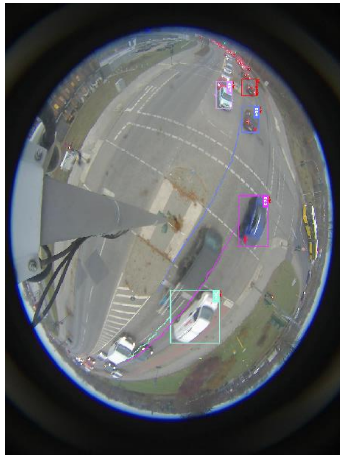
Figure 53: Object detection and tracking for the single sensor hemispheric camera Sony SNC-HM662 on a reference test site Berlin Ernst-Ruska-Ufer. Although the field of view is true 180° x 180°, the resolution in the image regions that correspond to 0° and 180° viewing angles is too poor for object detection.
