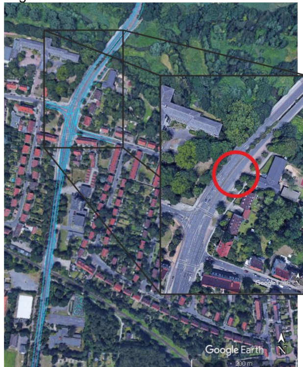
Figure 80: Tostmannplatz map showing the digital map (cyan) used by DLR vehicles. Test runs always started in at different places in the south for UC1-8. In the circle, the merging area important for UC5 is highlighted.
