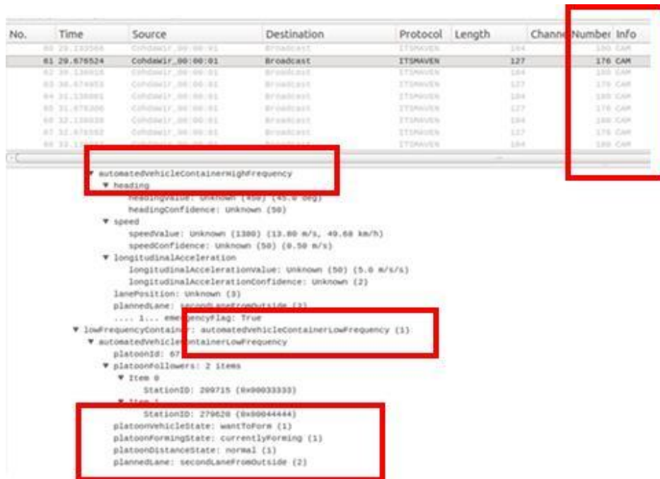
Figure 10: Logs of receiving V2X module
