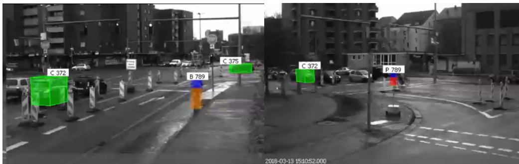
Figure 63: Abnormal trajectory: cyclist correctly classified (left), but later classification changes to “pedestrian” and object localisation has big errors (right).
