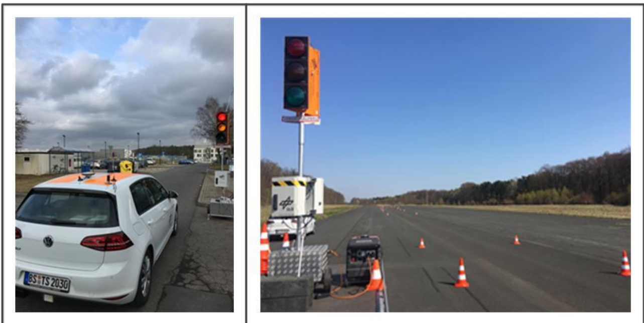
Figure 21: Mobile traffic light located on the DLR test track in Braunschweig (left) and in Edemissen (right), here adapted for the straight virtual road layout
