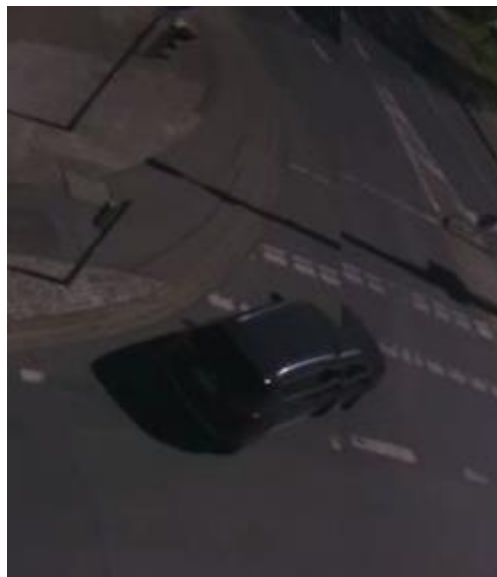
Figure 52: Image stitching artefact of PNM 9020V
