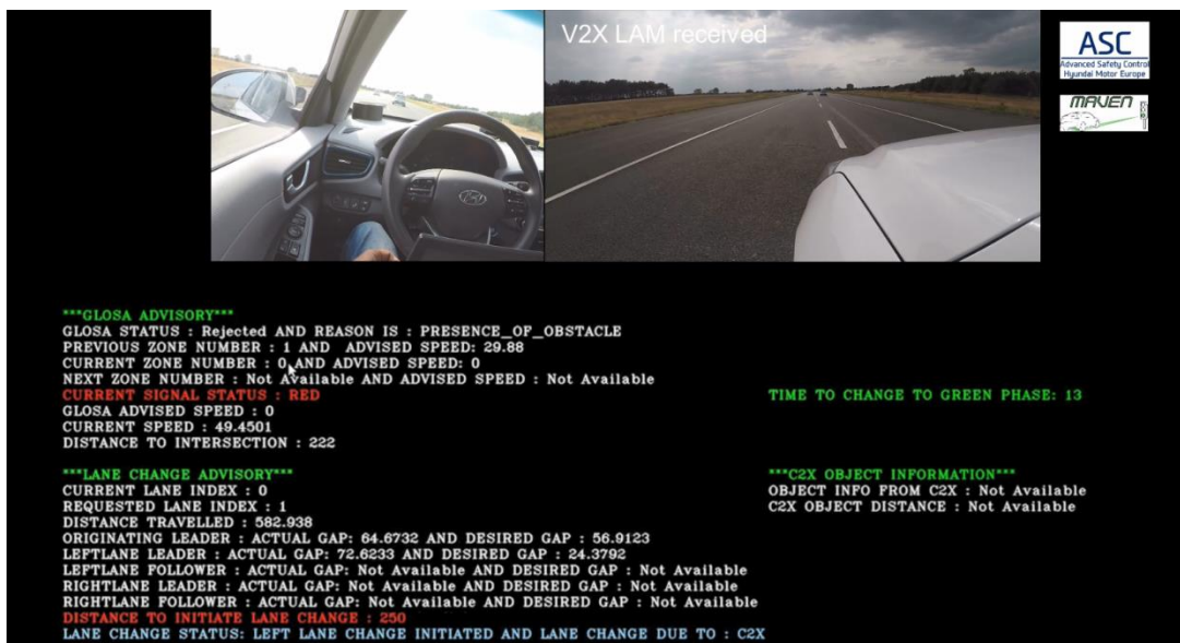
Figure 37: Test execution of automated adaptation to GLOSA and lane change advices (UC7 and UC8) at the HMETC car
