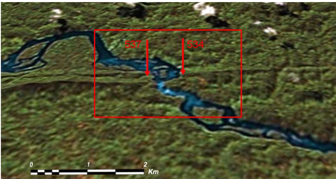
Fig. 9. 3D Landsat ETM+ image showing the ridge's elevations of 537 and 534m amsl taken as references for GIS digital lake reconstruction. (Image Landsat ©USGS, with additions.)
