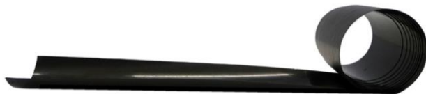
Fig. 2-15: Side view of partially coiled tape spring [29]
