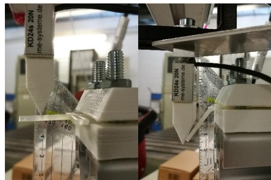
Fig. 5-7: Initial state and end of ≈ 55° bending during Test 1
