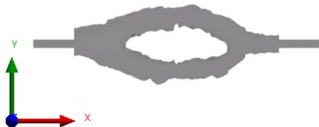
Fig. 3-14: Result with initial hole for a mass restriction of 8% of the initial mass
