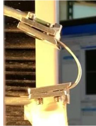
Fig. 2-45: Worst case gravity-induced sagging on CBT fixture [50]
