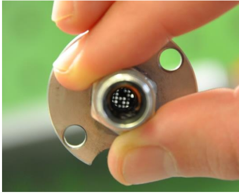
Figure 2: ADN-deposition after LMP-103S test; Clogged elements of \mu Showerhead injector.
