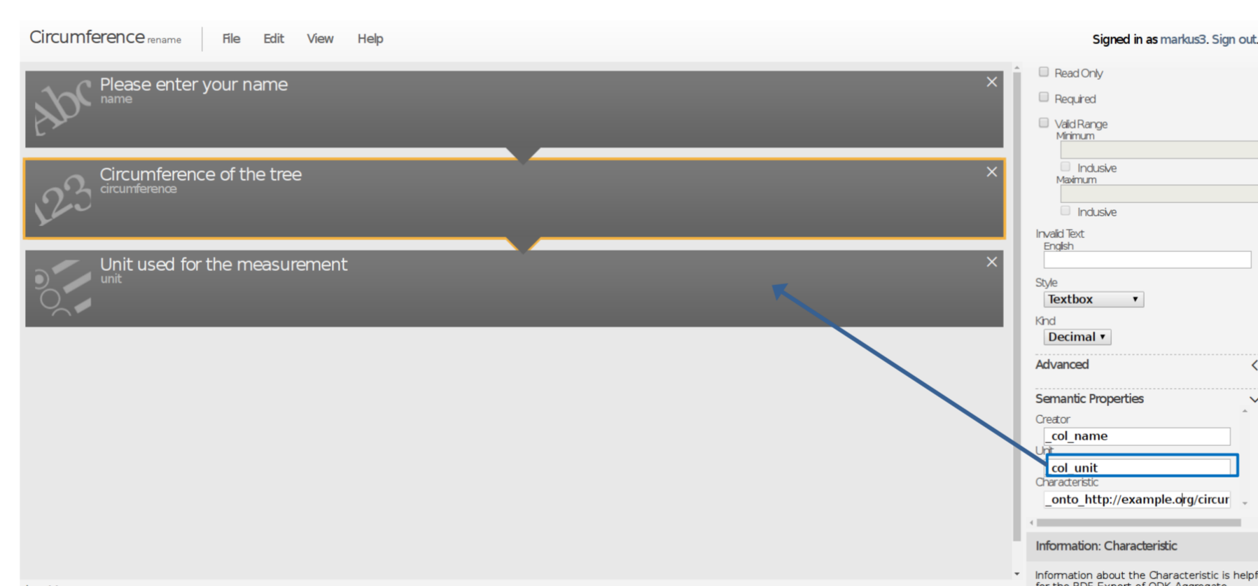
Metadata fields can be linked with form elements, e.g. the metadata information unit of measure for the input element tree circumference is linked with the unit selected via the single choice field unit.
