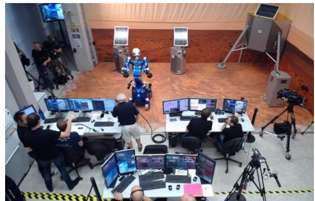
Fig. 9. The Simulated SOLar Farm EXperimental (Solex) environment. An assortment of smart payload units (SPU) and lander can be seen to be serviced, repaired, and installed by the robot Rollin' Justin
