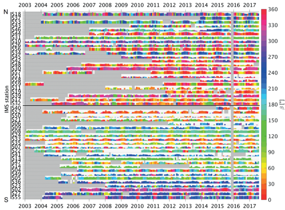
Figure 2: The monthly number of PMCC MAW detections is shown for all IMS station datasets available from the German National Data Center (HUPE, 2018). The stations are ordered from north (top) to south; the horizontal black line reflects the equator. The logarithmic scale indicates from 10^0 to 10^4 detections at each station. Colors code the monthly mean back-azimuths; gray boxes indicate missing data or the lack of PMCC results at the time of writing when the data from end-2015 were subject to reprocessing.
