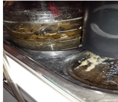
Fig.5 FOG accumulation on the top surface of solution in AMPTS bottle
