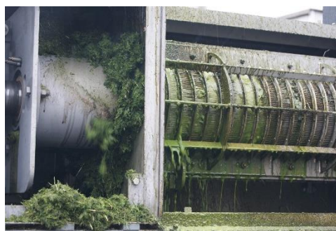
Figure 2: Screw pressing of fresh clover grass into green juice and press cake. Photo: Erik Fog, SEGES
