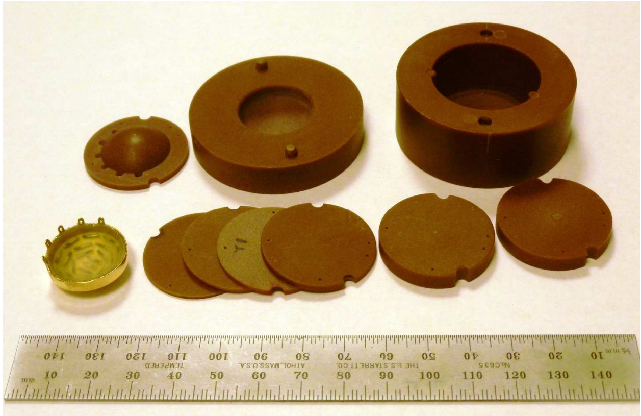
Figure 22. Solid Water "eye" phantom with its various inserts for measurements of the 20 mm COMS plaque with the fully loaded 20 mm COMS plaque at the bottom left corner.
