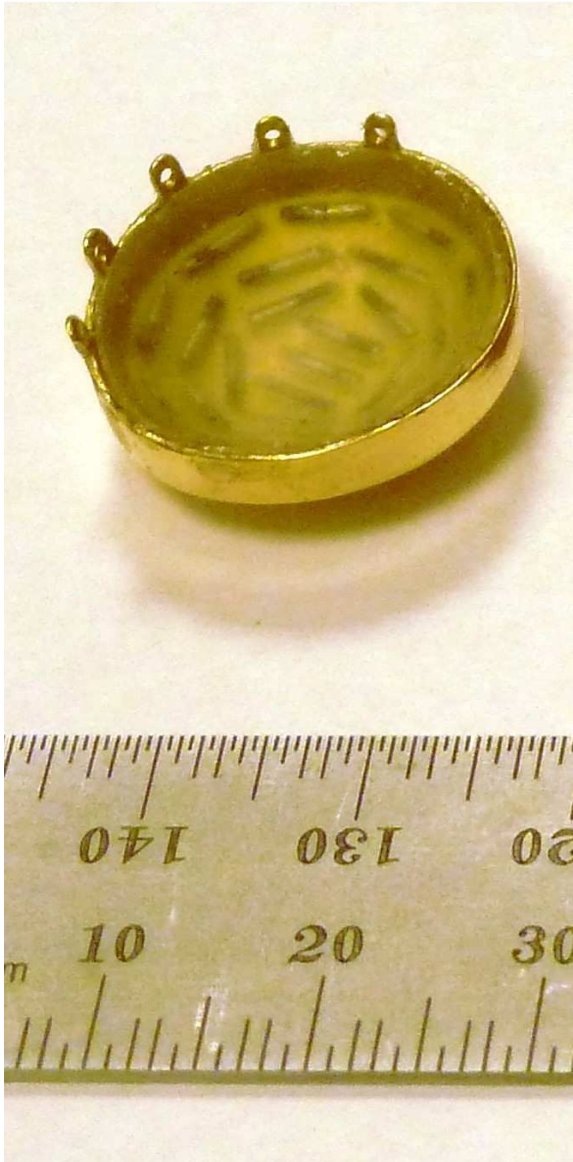
Figure 8. Picture of the fully loaded 20 mm COMS eye plaque dosimetrically characterized in this work. The Oncura 6711 seeds are visible through the silicone seed carrier. The ruler in the picture is a Starrett (L.S. Starrett Company, Athol, MA) metric ruler, with 0.5 mm smallest division.
