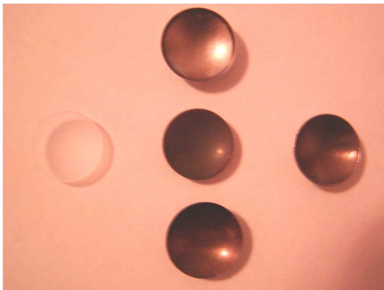
Figure 12. Second prototype quartz substrate before implantation (left) and after implantation with titanium encapsulation components (center), and after encapsulation in titanium (right).
