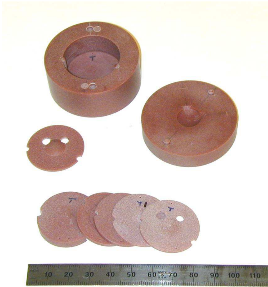
Figure 16. Parts of the “eye” phantom configured for a CCX plaque.
