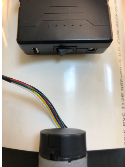
Figure L-3. Power connector and switch above motor.
