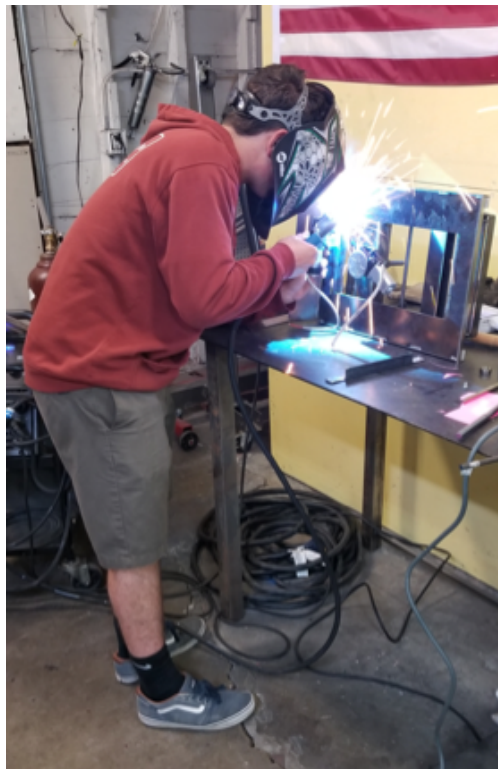
Figure 29: Photo taken of Alex welding components of the frame together
