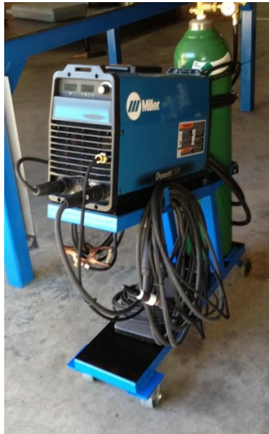
Figure 27: Miller welder used for this project
