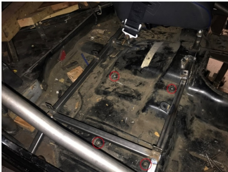
Figure 3. Floorboard Image Displaying the Uneven Design and Bolt Location
