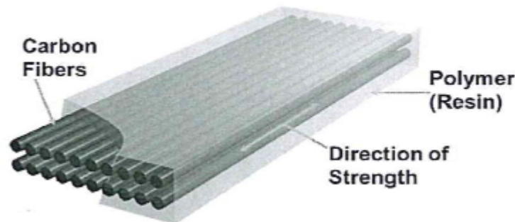
Figure 3.3 – Schematic Diagram of FRP Sheet [18]
