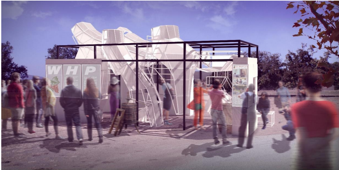
Figure 5: This is the team's final design intention. The black members are the added HSS superstructure to support the forms and wall. The form is built with \frac{3}{4} " steel tubing with polycarbonate paneling. The walls are wood framed with thermoplastic waterproofing
