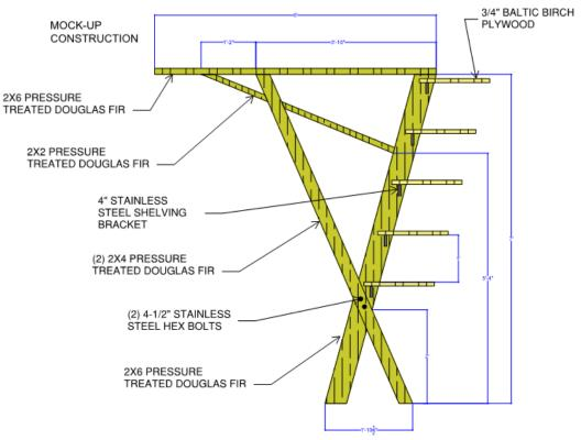
Figure 4: Construction drawing of our full scale model
