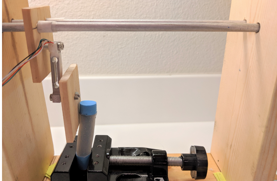
Figure 4.9: Un-jammed Fiber Jamming Chamber with 10mm Deflection
