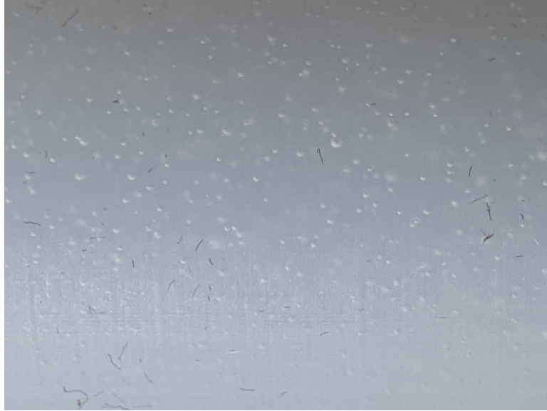
Figure 6.1: Bubbles present in all membranes manufactured
