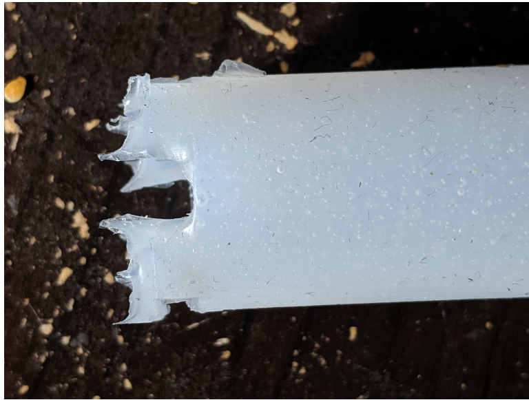
Figure 6.2: Slots left over after curing of membranes
