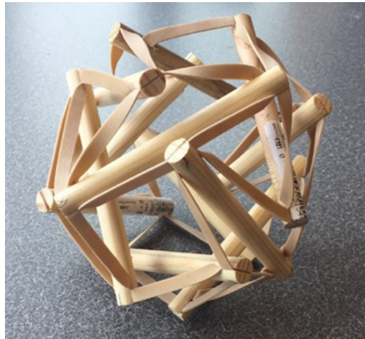
Figure 15. 12-Bar tensegrity structure concept model.
