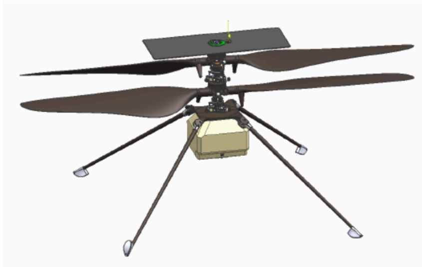
Figure 6. Mars Helicopter CAD drawing.
