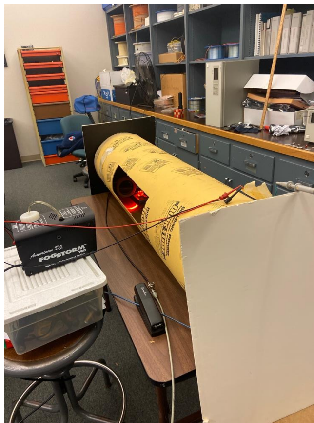
Figure 11: Test Set Up with Fog Chamber and Fog Machine
