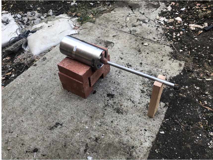
Figure 15. Final mini-keg gasifier model for testing
