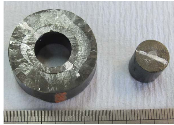
Figure 1. A photograph of the single grain GdBCO ring-shaped sample and a 12 mm diameter single grain cylindrical (core) sample.
