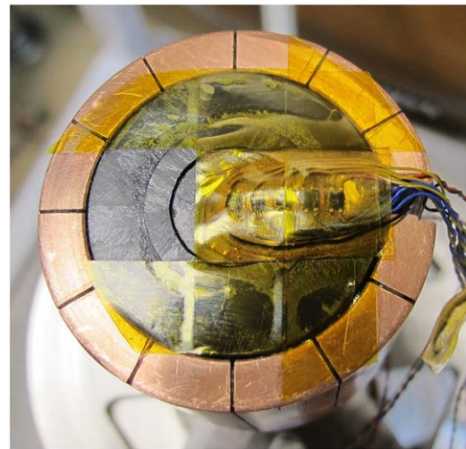
Figure 2. Sample assembly arrangement. Three Hall sensors are positioned on the inner core, and two sensors are on the ring. The distance between adjacent sensors is 2.5 mm. A further sensor is placed inside the bore of the ring.
