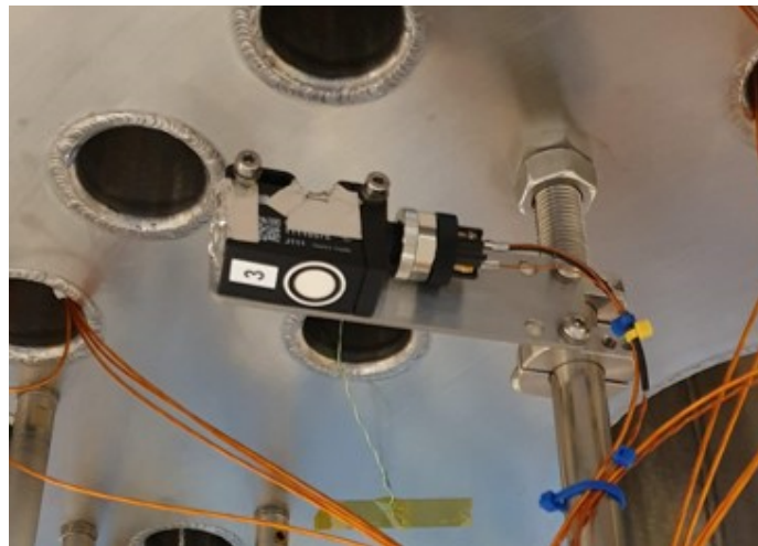
Figure 19: One of the three Baumer Ultrasonic sensors that are used to measure the flatness and fill level of LAr within the ARIADNE cryostat. All three are mounted at the same height - a few centimetres below the underside of the top flange.
