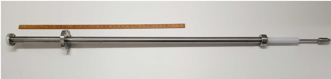
Figure 9: The ARIADNE high voltage feedthrough. A 1 metre rule is shown for scale.
