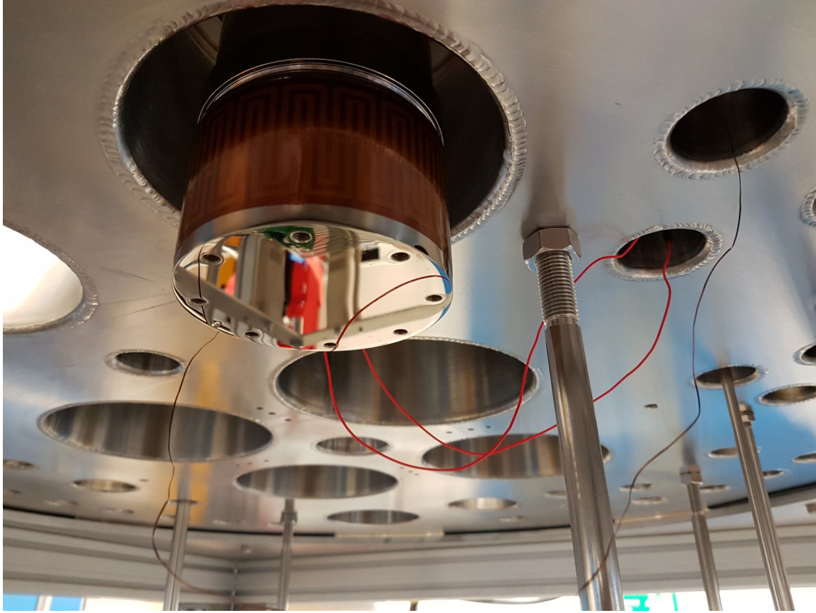
Figure 20: The Cryomech AL300 cryorefrigerator cold head extending down from the top flange of ARIADNE. A flexible kapton heater element wrapped around the cold head regulates cooling, and thus allows the pressure in the cryostat to be accurately controlled.
