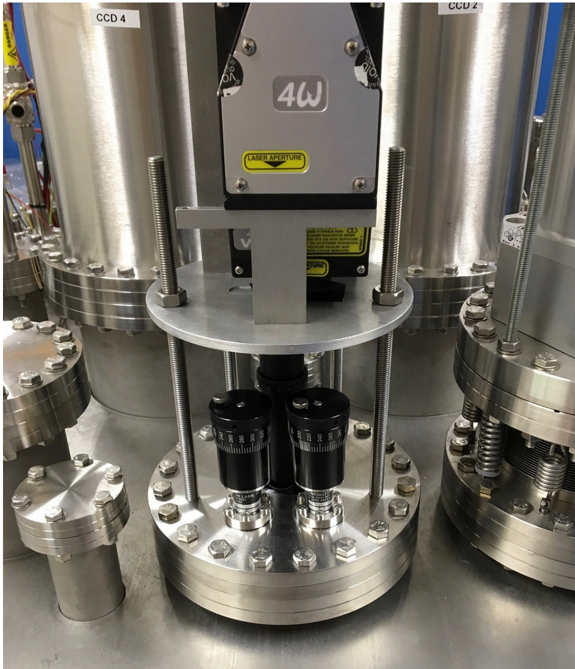
Figure 21: The Quantel Q-Smart 100 pulsed Nd:YAG laser, mounted on the top flange of the ARIADNE cryostat, together with the two rotary feedthroughs for controlling the position and orientation of the UV mirror.
