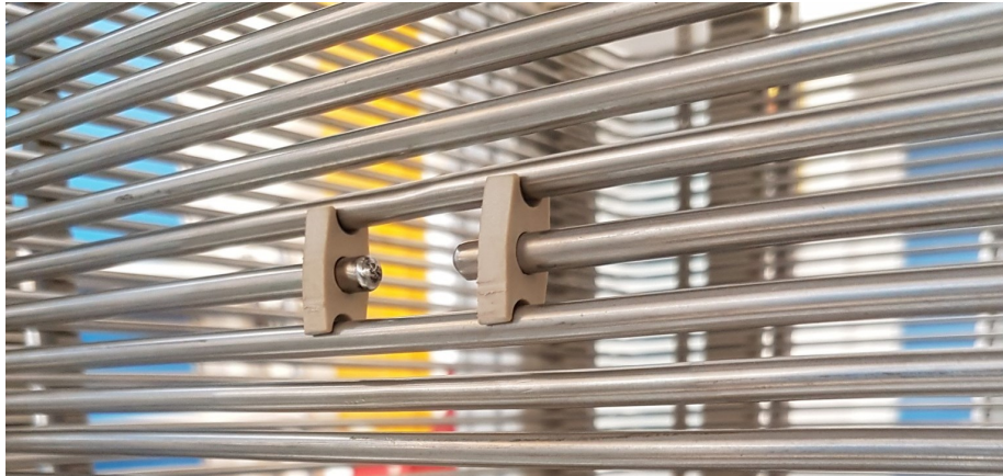
Figure 23: One of the eight small-width gaps in the TPC. The cut ends of the field-shaping ring have been smoothed and polished, to remove any sharp edges that might affect the drift field, and the gap is supported by PEEK elements.
