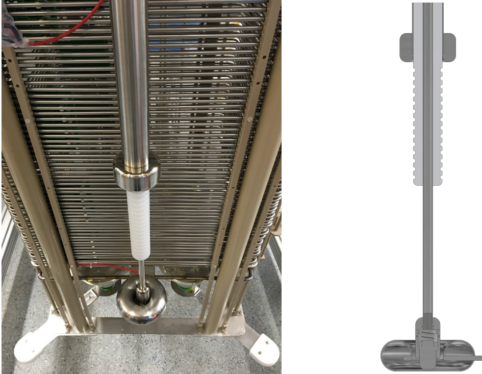
Figure 10: (Left) The ARIADNE HV feedthrough in-situ on the TPC, with the spring-loaded tip sitting within the cathode grid torus. (Right) A cross section of the lower end of the HV feedthrough.
