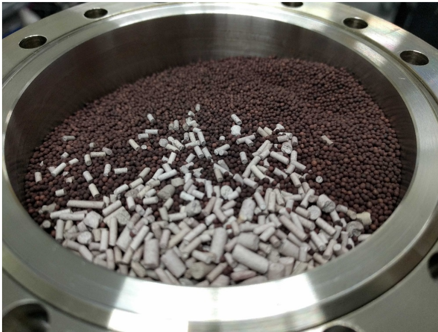
Figure 16: The external 30 L filtration cartridge, showing the mixture of 85.6% Engelhard Cu-0226 S 14 × 20 (brown balls) and 7.2% of both 3 Å and 4 Å molecular sieves (white cylinders in two different sizes). The same mixture is present in the internal 13.5 L cartridge.
