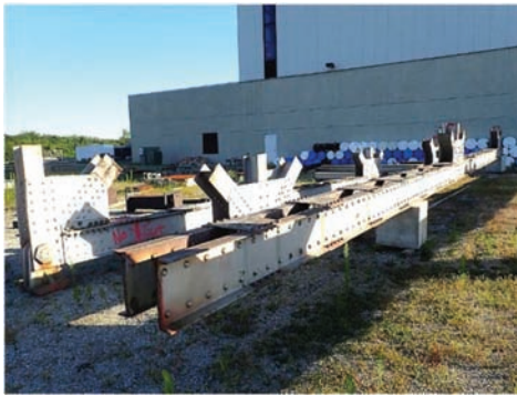
Figure 1.1 Winona Bridge Specimens as they arrived.
