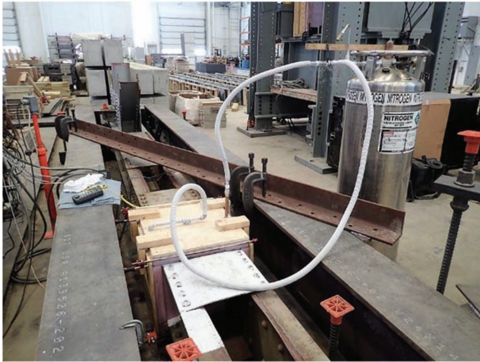
Figure 4.3 Cooling chamber used to cool section of Specimen 2 prior to testing.
