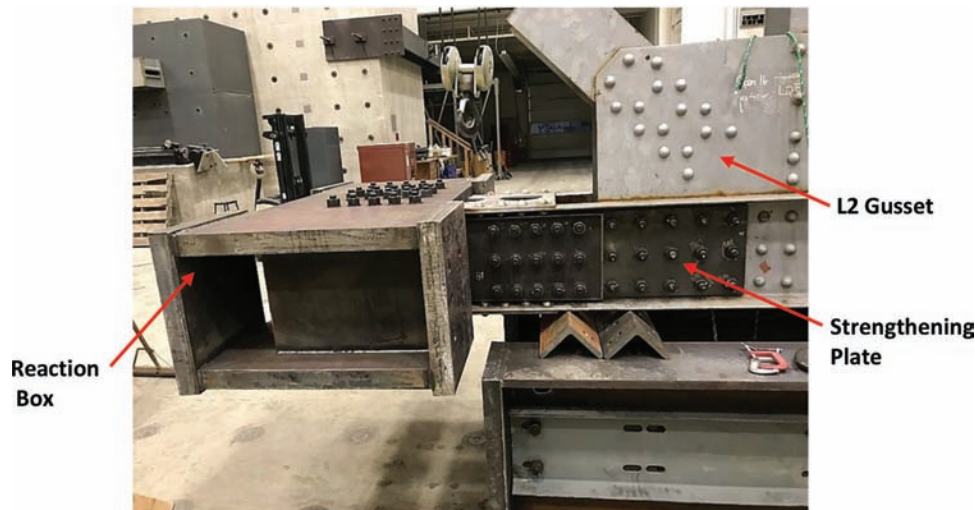
Figure 3.6 Connection at the reaction end of the specimen showing the additional plate added to allow for strength testing of the main section of the specimen.
