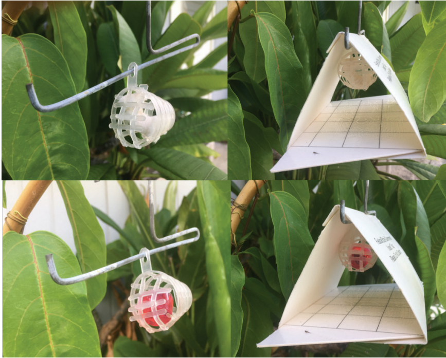
Figure 1. Standard method of baiting Jackson traps. Top row: Cotton wick containing ME in perforated basket and basket positioned inside Jackson trap. Bottom row: Polymeric plug containing TML in perforated basket and basket positioned inside Jackson trap.
