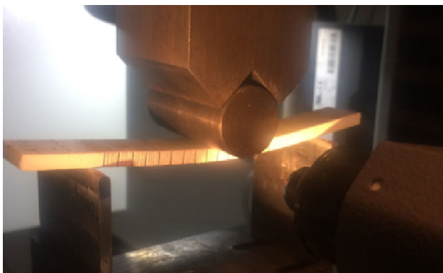
Figure 11 ENF test set-up with a scale ruler marked face. A travelling microscope was again used for measuring the crack length.
