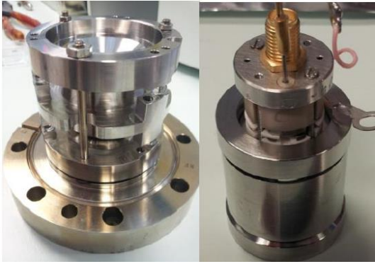
Figure 2: (left) High-speed (right) low-speed deployable Mass Spectrometer instruments
