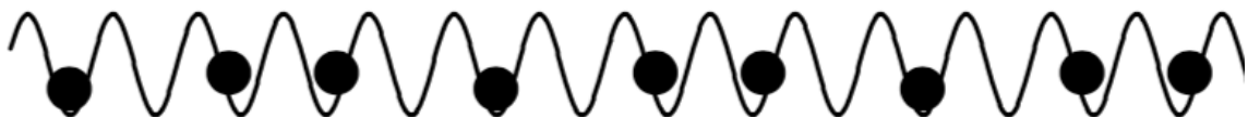
Figure 2.4: Ground state arrangement for \theta = 3/5 where 3 particles are located within a periodic region of length 5a_{CE} . Figure taken directly from Fig. 5.3 in [2].
