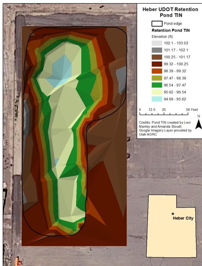
Figure D6. TIN surface representing the interior topography of the Heber retention pond.
