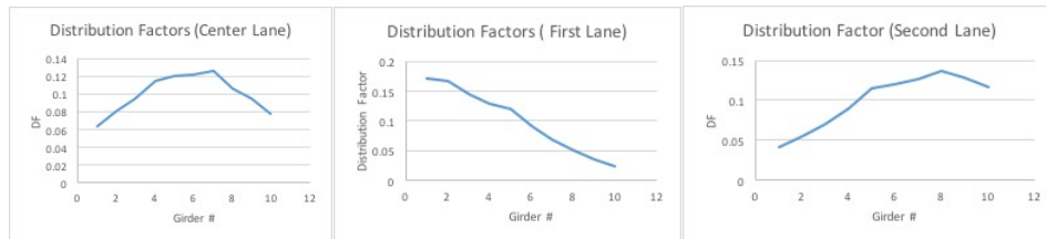
Fig. 17. Girder Distribution Factors based on measured strains in the midspan depending on the transverse position of load
